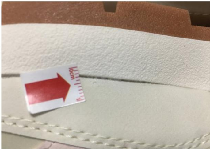
07 Defect-Glue mark on the surface-mi
