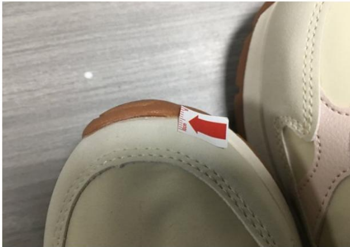
01 Defect-Lack glue at the shoe toe-ma
