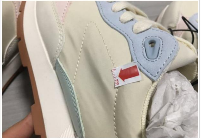
02 Defect-Waving at the upper surface-ma
