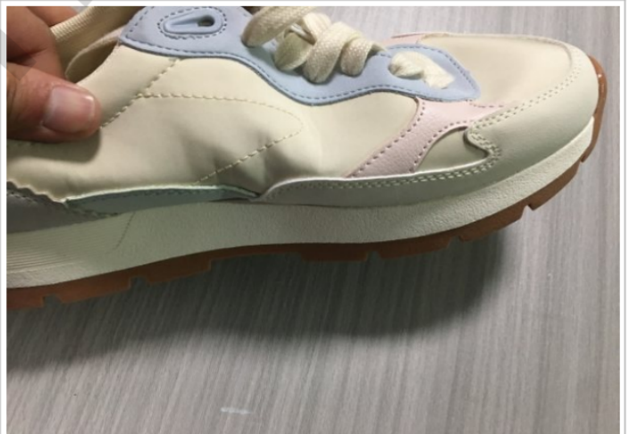
30 Flexing test on the outsole
