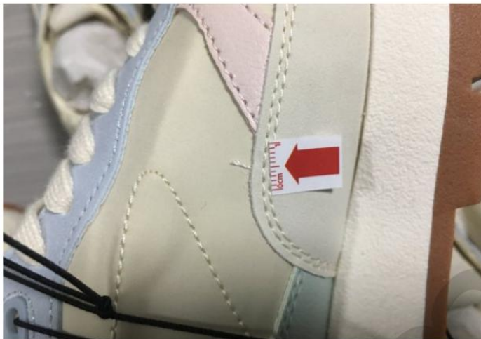
03 Defect-Uncut long thread end-mi
