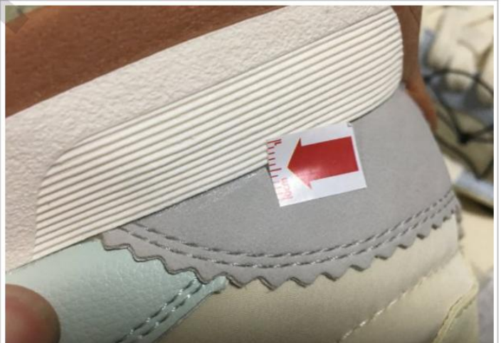
06 Defect-Glue mark on the surface-mi
