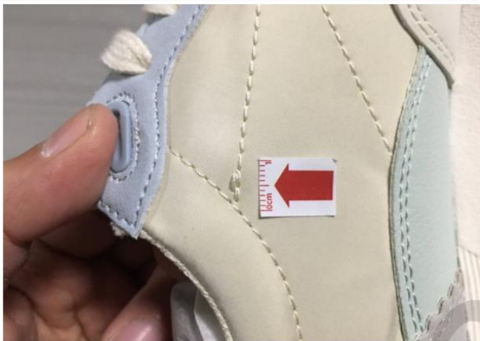
09 Defect-Poor stitching at the upper surface-mi
